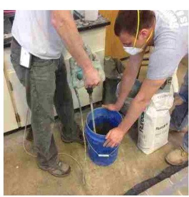
Preparing cementitious matrix
