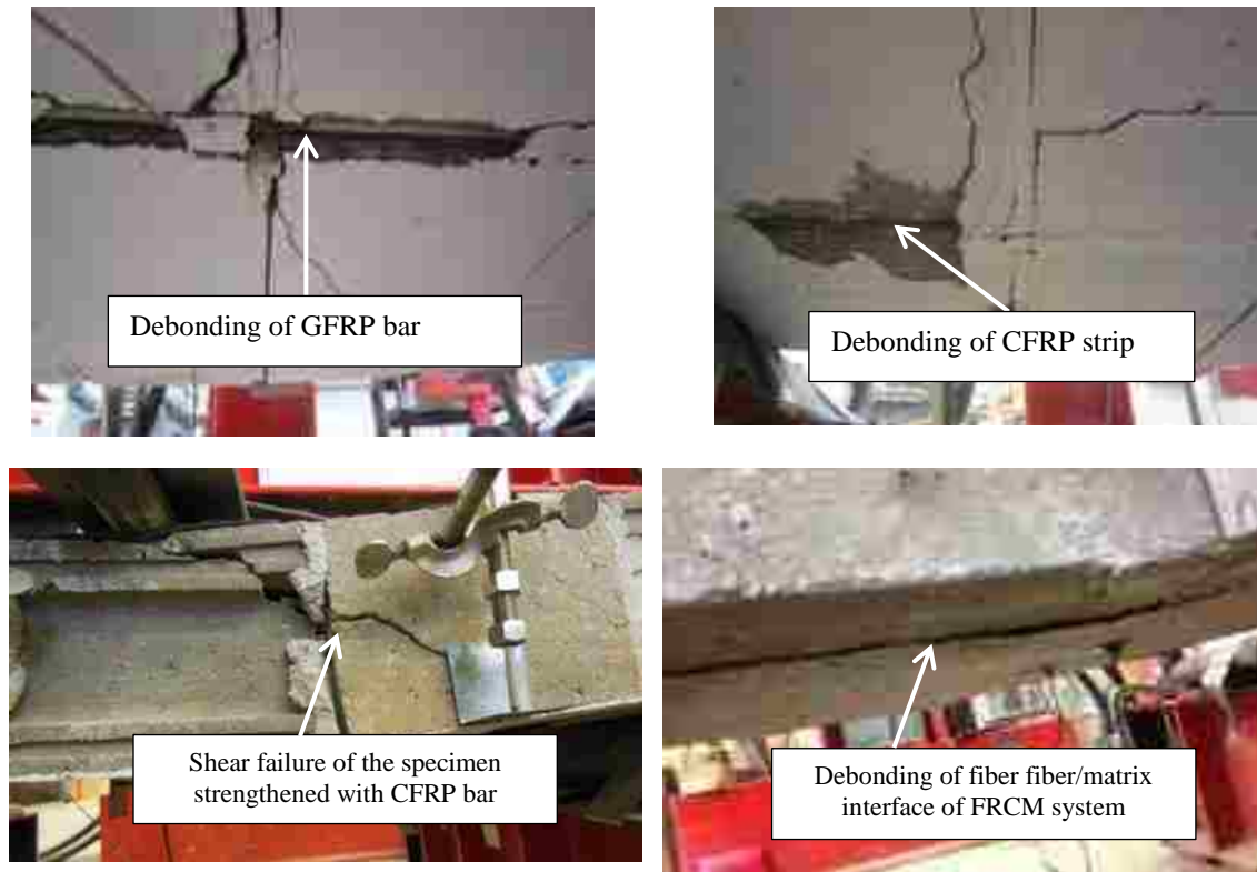
Figure 13. Observed modes of failure
